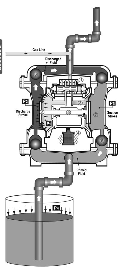
Gas-Operated Double Diaphragm pumps are powered by compressed gas, nitrogen or natural gas.
