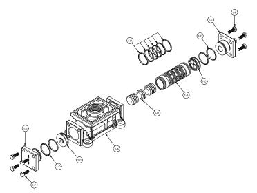
**Valve Assembly for Aluminum Mid Sections**
