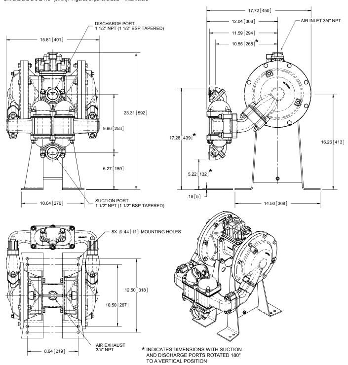
Model HDB1 $\frac{1}{2}$ -A features 1 $\frac{1}{2}$ " NPT threaded connections. Model HDB40-A features 1 $\frac{1}{2}$ " BSP Tapered connections.
