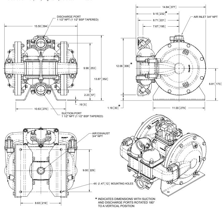
Model HDB1½-A features 1½" NPT threaded connections. Model HDB40-A features 11/2" BSP Tapered connections.
