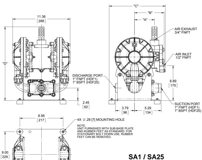
HEAVY DUTY FLAP VALVE PUMP BOTTOM PORTED DIMENSIONAL TOLERANCE ±1/8 [3] [XX] = MILLIMETERS
