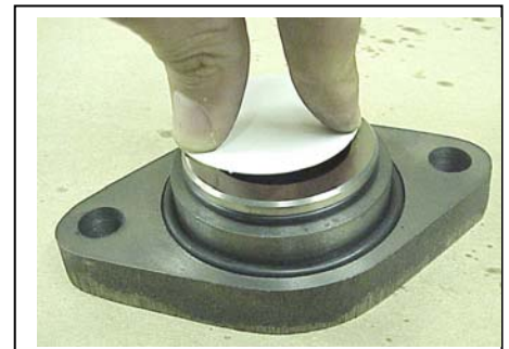
Figure 19, Stationary set install
