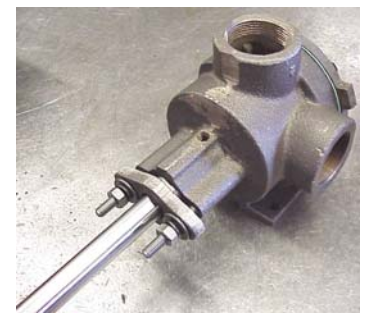
Figure 11, Gland & fasteners installed
