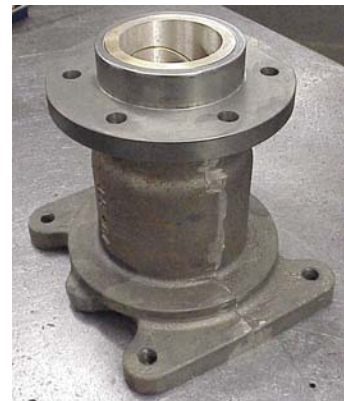
Figure 7, The RBS bushing installed
