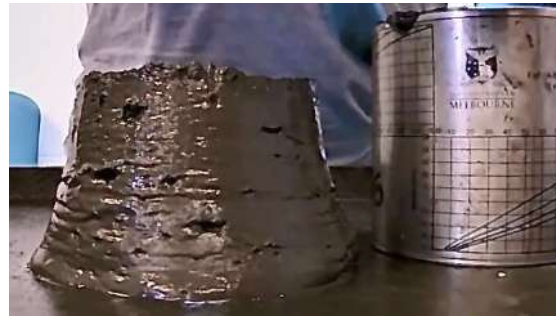
Slump test, solid content > 75%
