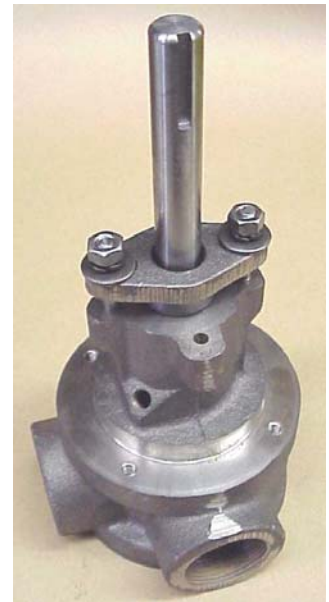
Figure 9, Gland & shaft installed
