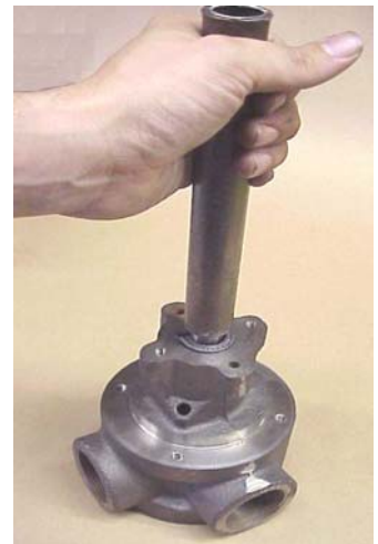
Figure 8, Pushing in the packing rings
