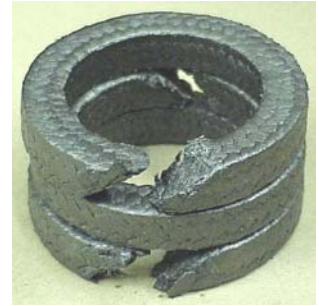
Figure 7, Alternate the packing cuts
